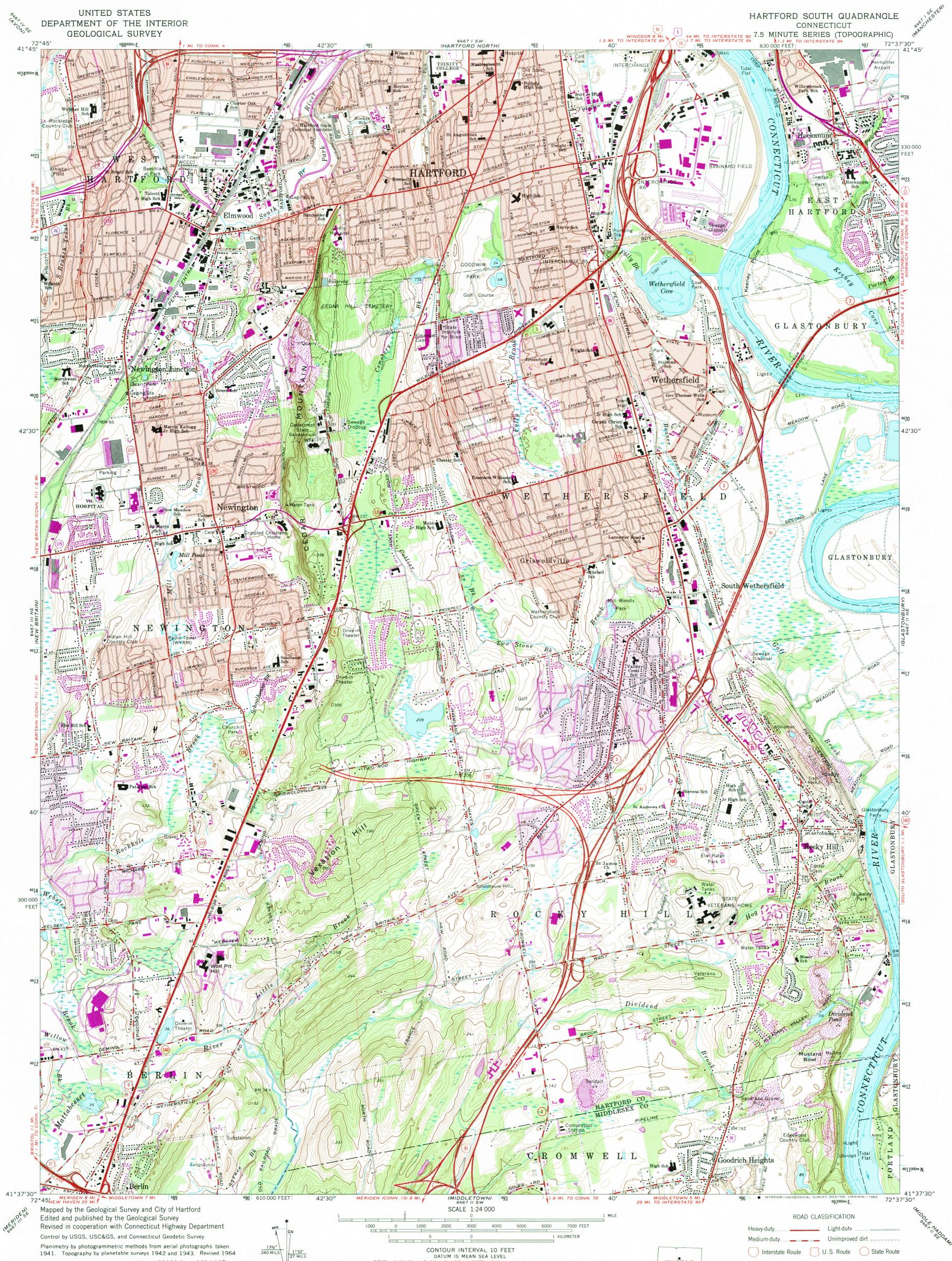
Planimetry by photogrammetric methods from aerial photographs taken 1941. Topography by planetable surveys 1942 and 1943. Revised 1964
